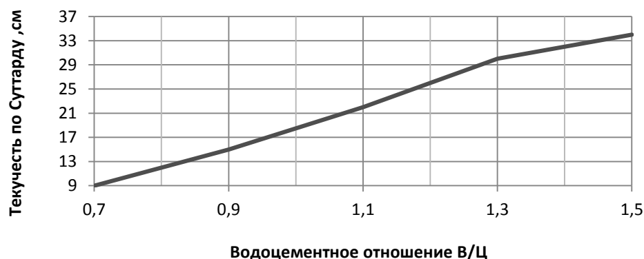
Fig. 1. The dependence of the fluidity of foamed concrete mixture based on perlite from water-to-cement ratio
